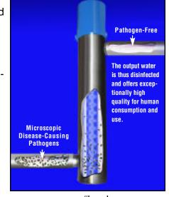
For maximum UV transmission a "hard glass" quartz sleeve is recommended for two main reasons. It isolates the lamp from the water to offer more uniform operating temperatures and allows for higher UV output into the water.
